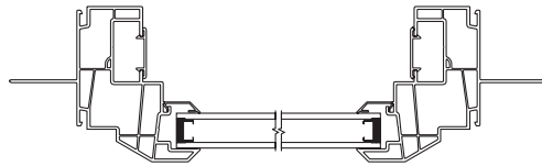
Single Hung Studio Window – Horizontal Section
